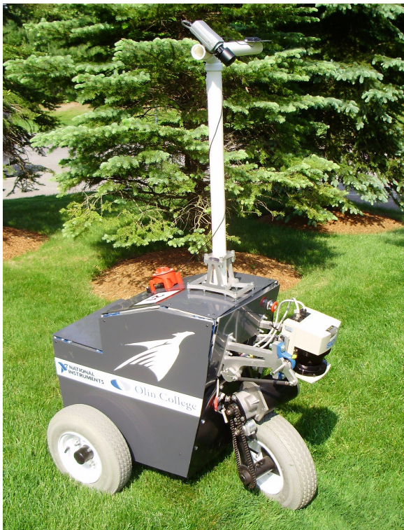
Figure 1: Photograph of Athena. Pictured is the Franklin W. Olin College of Engineering 2010 IGVC entry. Athena brings together several computing fabrics to implement a true subsumptive architecture.
